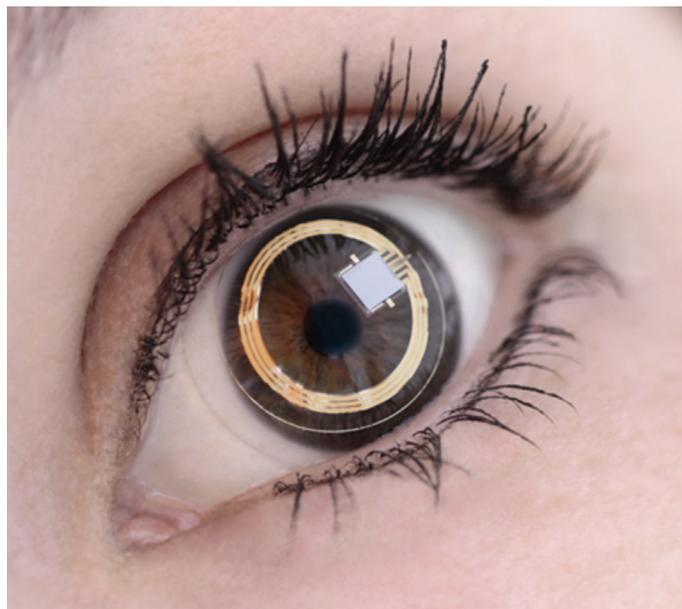
*Soft silicone contact lens with intelligent elements, such as strain gauges and an application-specific circuit embedded.*
